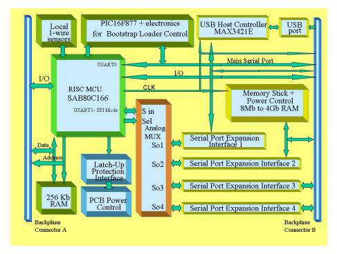
Figure 3. Preliminary block diagram for the PDS computer.
