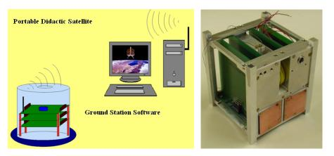
Figure 1. Fundamental parts of the POSTSAT.
